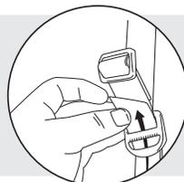
Thread strap through mounting point and back through same slot in thumb-lock buckle.
