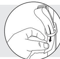
Thread strap thumb-lock buckle and pull to tighten. Remove straps from unused mount points (but use all 3 if possible).
