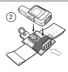
Slide the Garmin Mini Spine Mount Adapter under the webbing strap.
